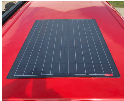
This semi-flexible panel from NDS is ideal for pop-top roofs on campervans where there's a slight curve.
